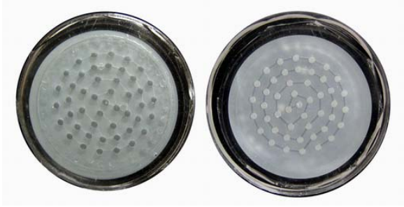
Fig. 2 Completed multi-DNA extraction device.
