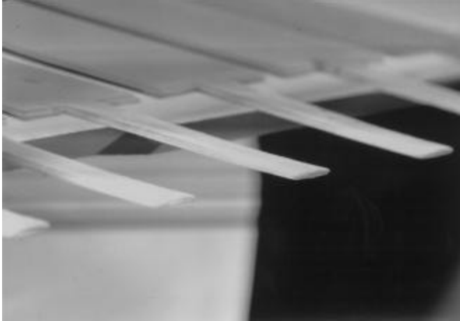
Figure 4. Scanning electron micrograph of a micromachined pipette array. The wide sections are 12750 \times 1500 \times 30 \mu\text{m}^3 (L×W×H). The microchannels extend 1.5 mm from the silicon substrate and are 500 \mu\text{m} wide. The structural material is electroformed nickel with wall thickness of 15 \mu\text{m} .
