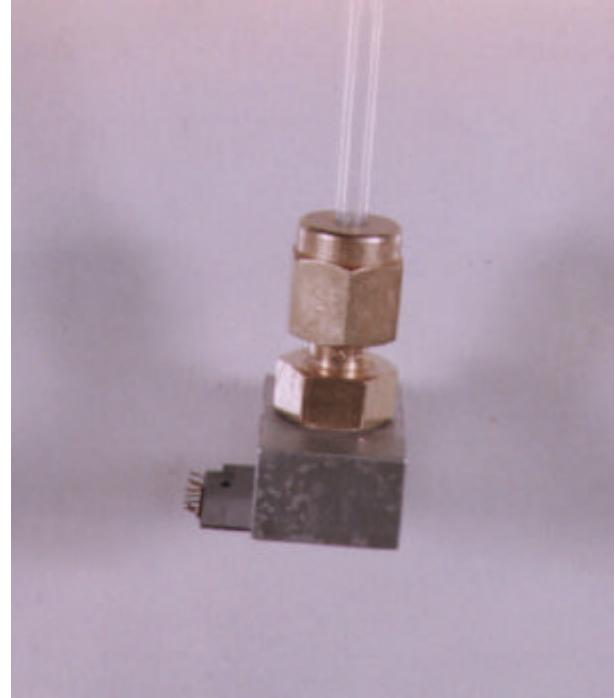
Figure 6. Photograph of a micromachined pipette array interfaced from the back side. A 1/8 in tubing and 1/8 inch swagelock adapter are used to connect micro-interface to the macro pressure source
